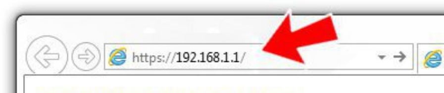
Figure 25: Entering the IP address of the router
