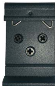
Figure 9: Default position of DIN rail clip
